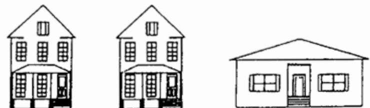
Directional Emphasis - Inappropriate: Shown here are two historic houses, each with a vertical directional emphasis, and a new house that is clearly horizontal in emphasis. This new building is not sympathetic nor consistent with the established pattern of directional emphasis along this street.
